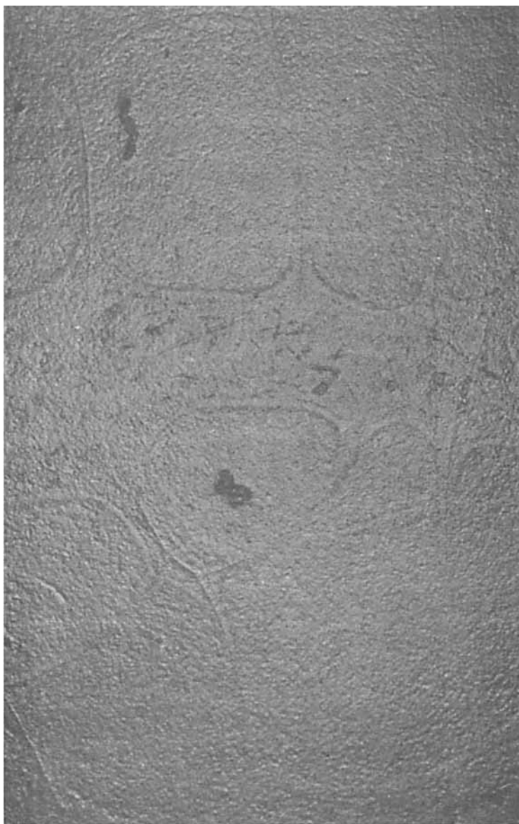
Fig. 13. Micrograph from PVAc of 0.041 \times 10^6 and PEMA of 4.48 \times 10^6 (40% PEMA) (magnification of 25).
