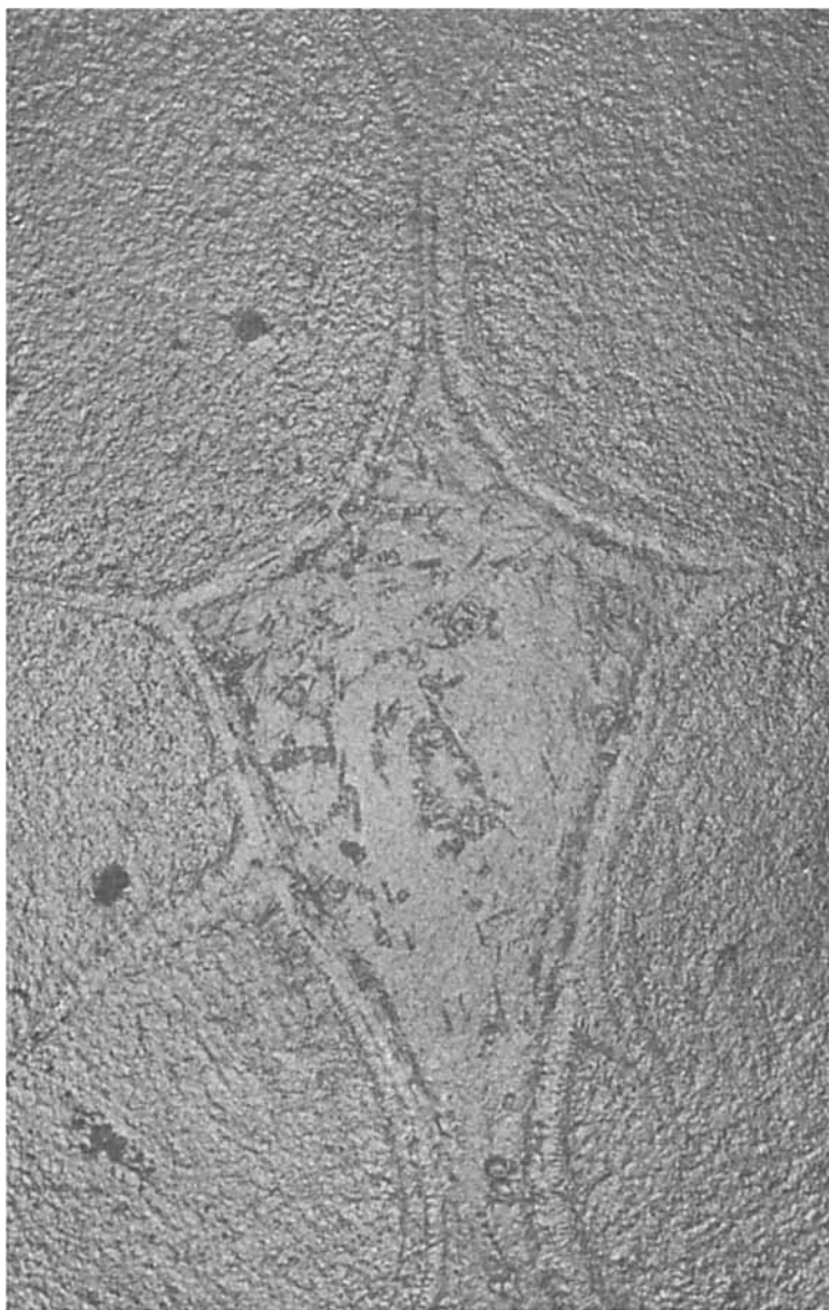
Fig. 9. Micrograph from PVAc of 0.46 \times 10^6 and PEMA of 0.89 \times 10^6 (40% PEMA) (magnification of 25).
