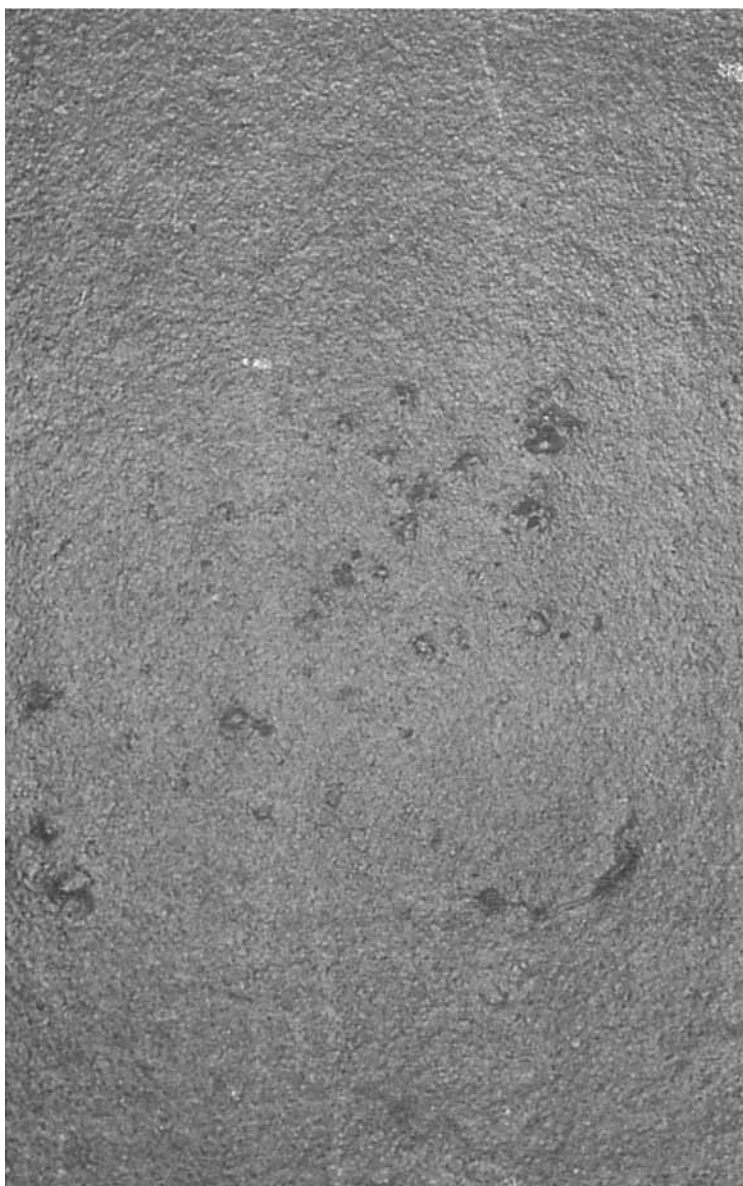
Fig. 14. Micrograph from PVAc of 0.041 \times 10^6 and PEMA of 4.48 \times 10^6 (80% PEMA) (magnification of 25).
