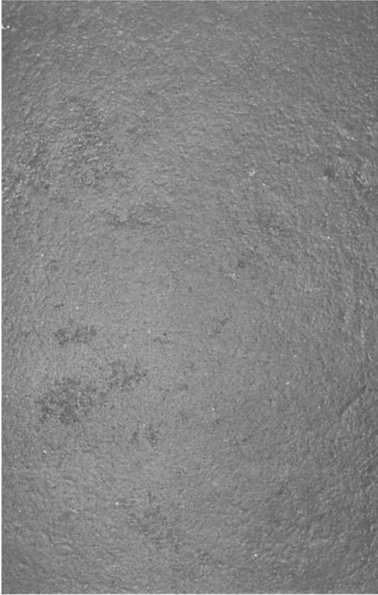
Fig. 15. Micrograph from film used for Figure 12 heated in an air oven at 100°C for 1000 h (magnification of 25).
