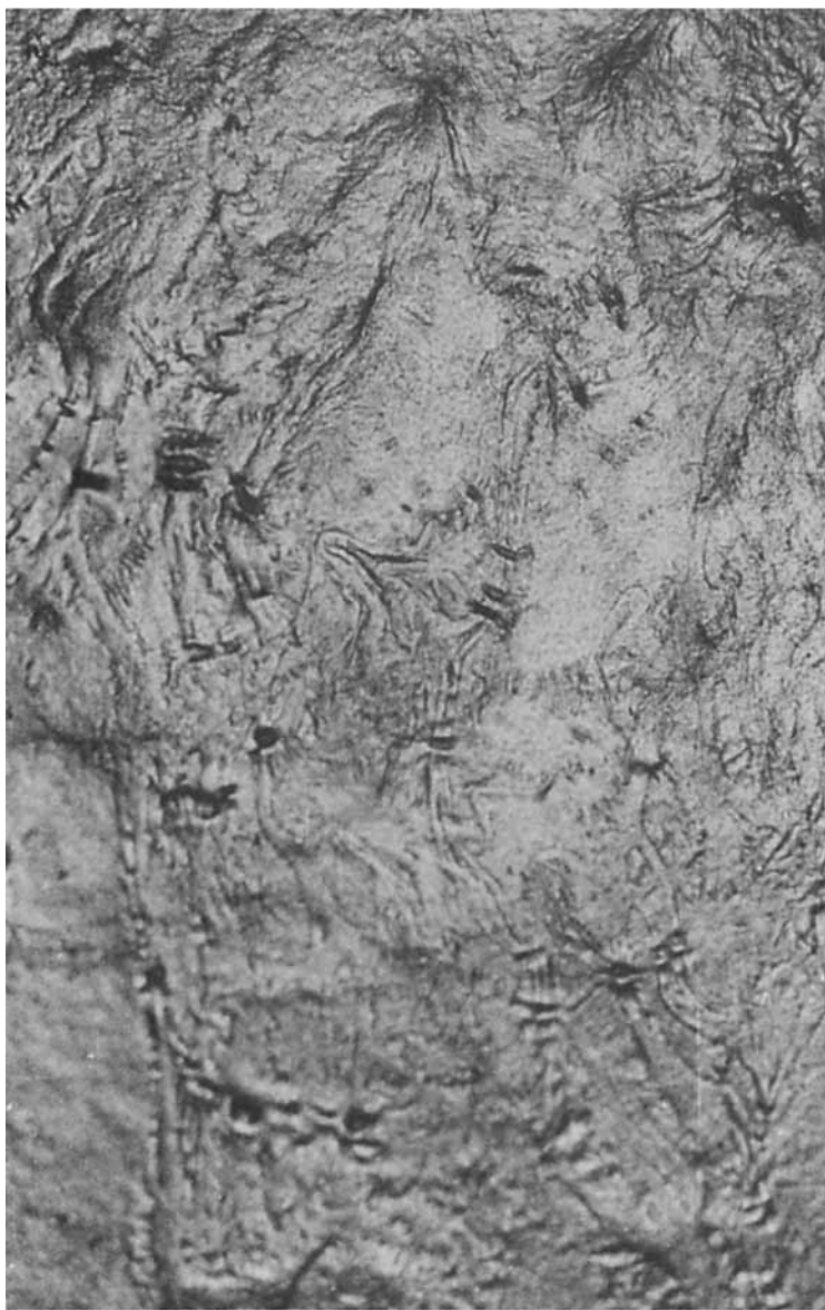
Fig. 11. Micrograph from film used for Figure 8 heated in an air oven at 100°C for 1000 h (magnification of 25).
